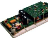
A high reliability laser charging power supply, for tactical target designation equipment, with a capability for either local or remotely controlled operation.
