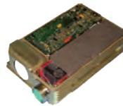
High and Low Voltage Power Supplies for the pilot helmet system on the Tiger Attack Helicopter, converting 28Vdc Avionics into multiple outputs in a high vibration environment.
