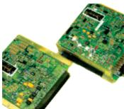
Multiple output low voltage power converters for use in multifunction displays fitted to the Hawk Fighter Trainer aircraft, built-in-test, with variants for 28Vdc and 115Vac inputs.
