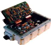
High reliability power supplies designed to withstand the highest demands of mobile battlefield operations, powering imaging systems, GPS navigation and communications equipment.
